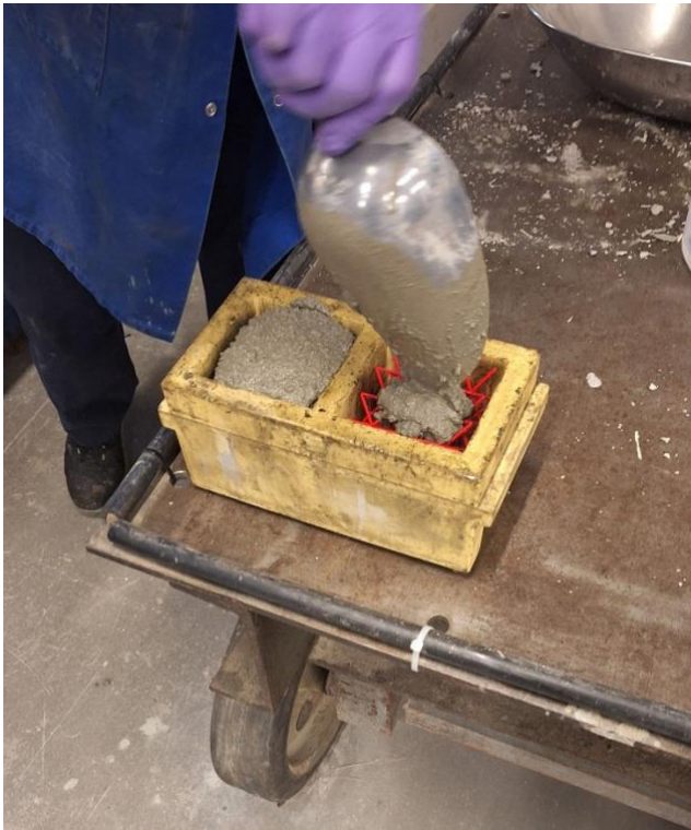
Figure 7. The process of moulding of PLA lattice-reinforced cementitious specimens
